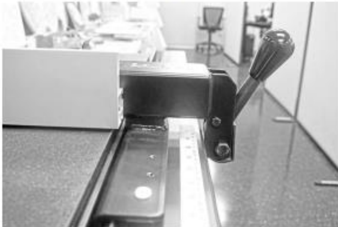
Fence fitted over the front guide rail
