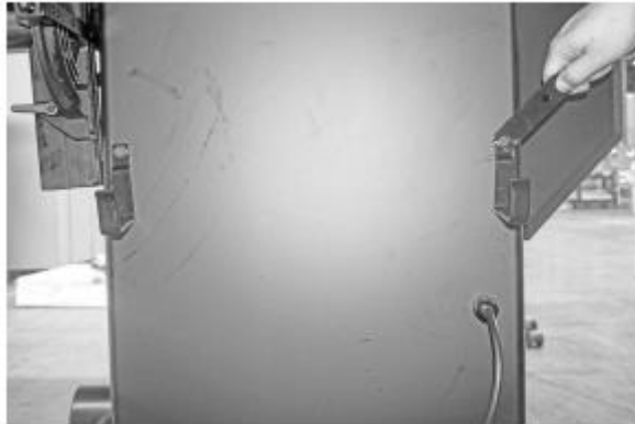
Fence Hook Installation
