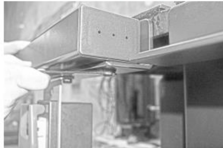
Attaching the left front rail body to the left front rail using the shorter hex bolts and flat washers.
