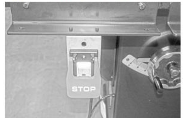
Control Switch correctly mounted. The expose bolts will fit the through holes in the fence body
